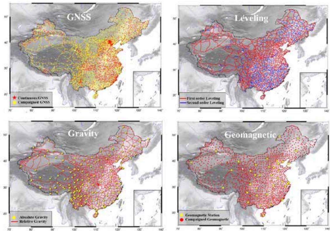
**Fig 3. Schematic Diagram Chinese Continent Integrated Geophysical Field Observation**
