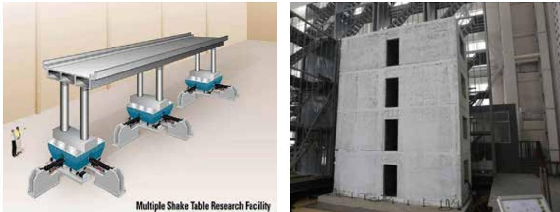
**Fig 9. Large-scale and Large-load Seismic Simulation Facilities**
