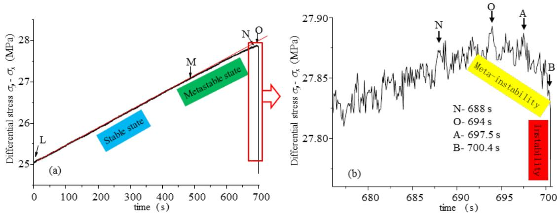
**Fig 6. The Curve of Differential Stress and Time**
