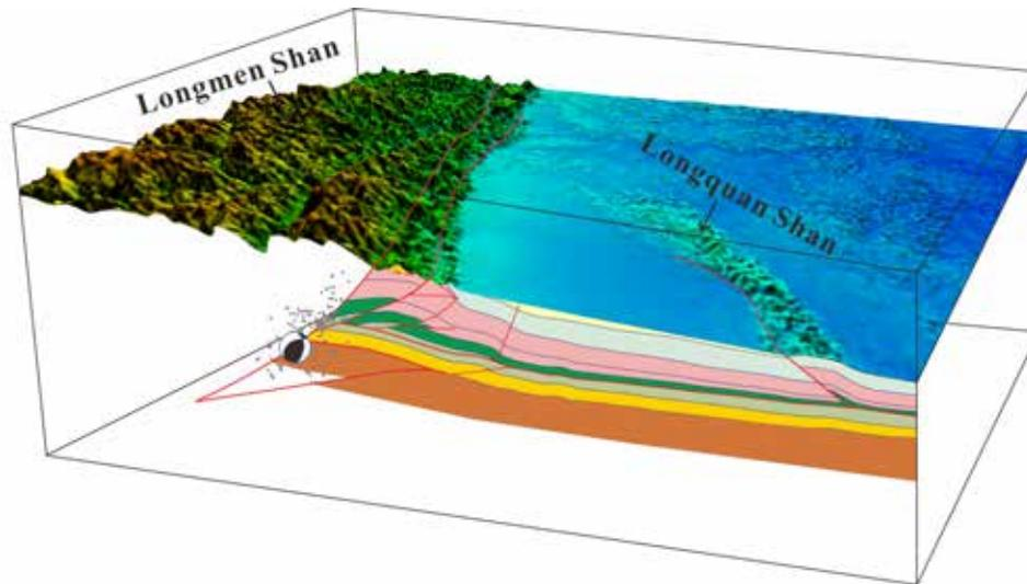
**Fig 5. Three-dimensional Structure of Crust and Faults in Longmenshan Area**
